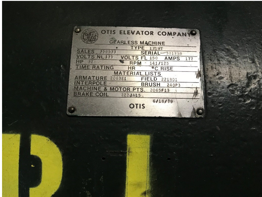
Car 1: Otis 131 HT name plate data tag.
